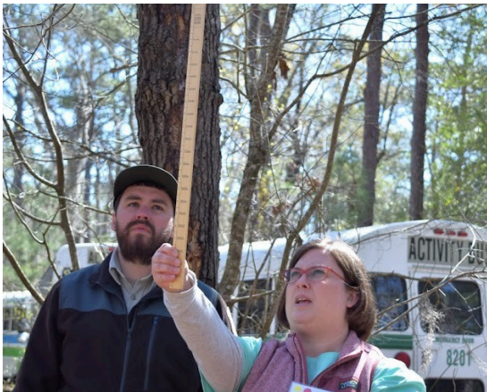
Katherine Alligood, advisor at Beaufort County Early College, uses a Biltmore stick to estimate tree trunk diameter.
